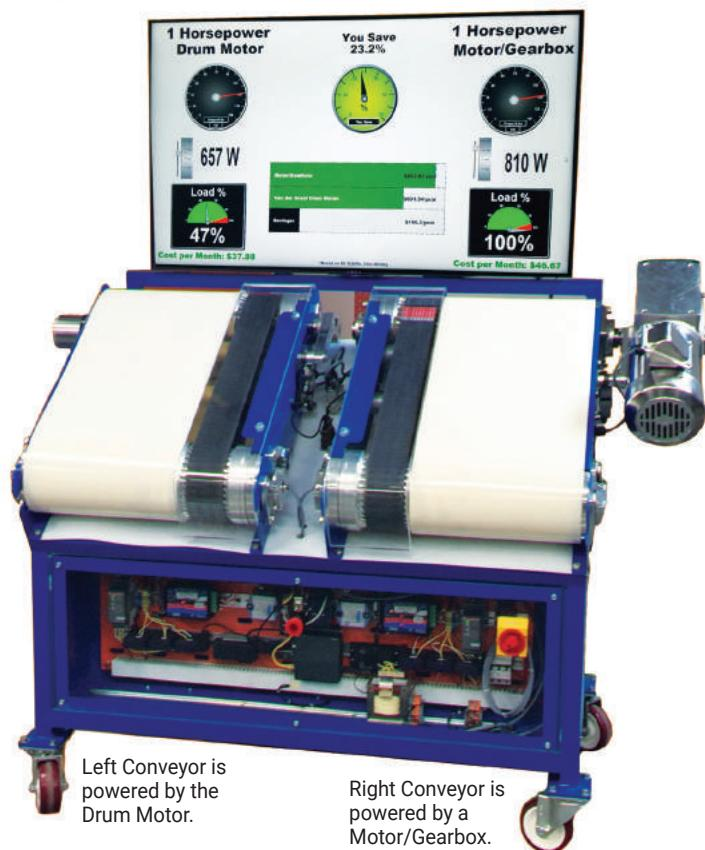
The tests revealed that the conveyor powered by the **VDG drum motor saves 23% energy** when compared to the conventional conveyor drive. The drum motor, while producing the same torque as the motor/gearbox, is operating at a fraction of its full capacity, extending the life span of the drive as well as reducing maintenance.
