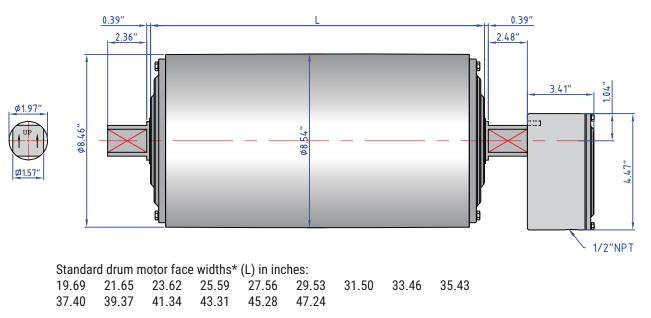
**NOTE**: Junction Box **does not rotate**. Power entry at 6 o'clock position.
