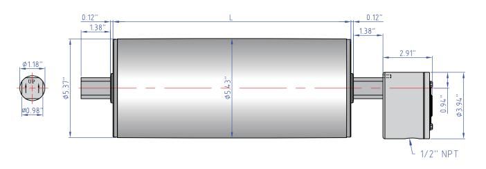
**NOTE**: Junction Box does not rotate. Power entry at 6 o'clock position.
