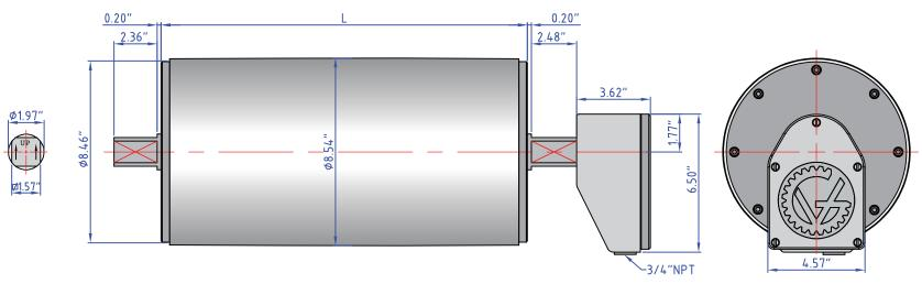
Standard drum motor face widths\* (L) in inches:
