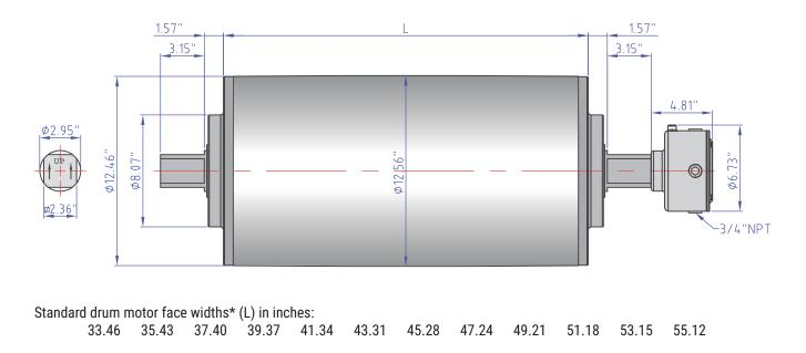
\*Some face widths are not available in all horsepowers. For minimum available face widths: <u>Click Here</u> to View Chart. \*\*Idler dimensions are identical to the drum motor with no junction box.
