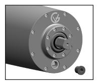
To verify the oil level, rotate the drum motor until the oil plug is in the 4 o'clock position as shown in the diagram. The minimum oil level
