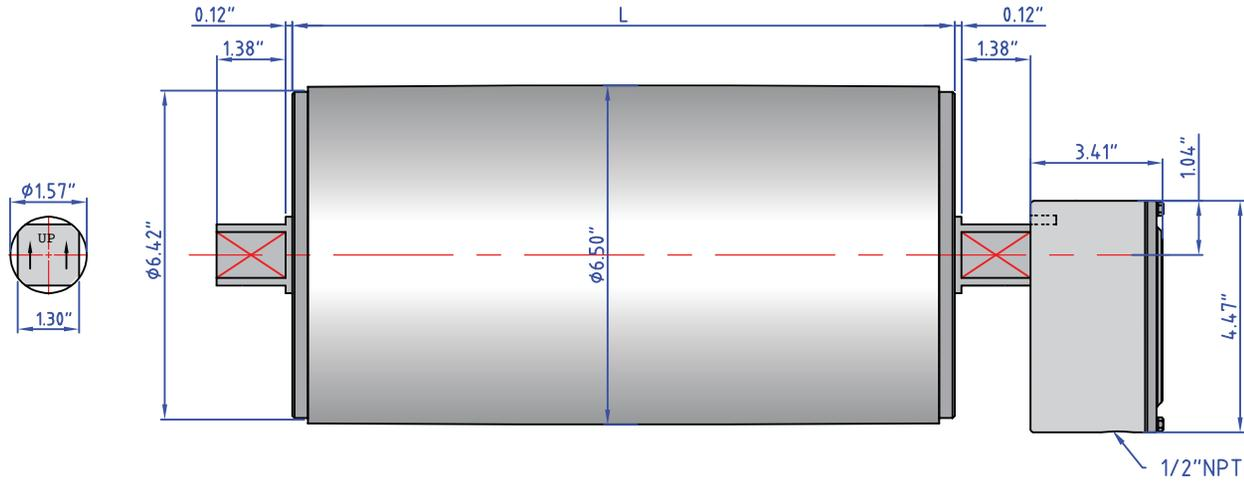
Standard drum motor face widths\* (L) in inches:
