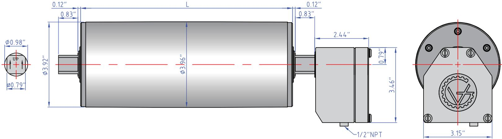
Standard drum motor face widths\* (L) in inches:
