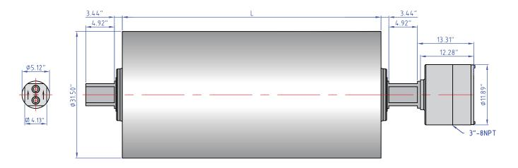
Standard drum motor face widths\* (L) in inches:
