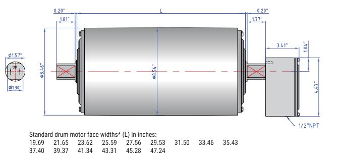
**NOTE**: Junction Box **does not rotate**. Power entry at 6 o'clock position.
