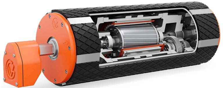
In order to achieve any heat transfer from the drum motor to the belt, the drum motor could not be covered with rubber lagging. However, most of the drum motors sold today are lagged with rubber, making it extremely difficult, if not impossible, to remove heat from the drum motor.
