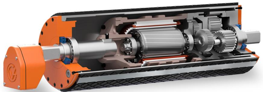
The input power cable passes through the hollow shaft and is connected to the motor stator. The electric motor is mechanically connected in-line to the gear reducer. The drum motor is partially filled with oil. The oil inside the drum motor lubricates all mechanical components and helps to dissipate heat generated by the electric motor and gear reducer onto the drum, and from the drum to the belt. In theory, the drum motor is cooled by the belt making full contact with the rotating steel drum.
