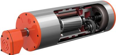
As the temperature inside the drum motor rises, the internal pressure can rise up to 1 Atm (atmosphere) or 14.6 psi. Because of this internal pressure, it is necessary for the drum motor to be hermetically sealed to prevent oil leaks.
